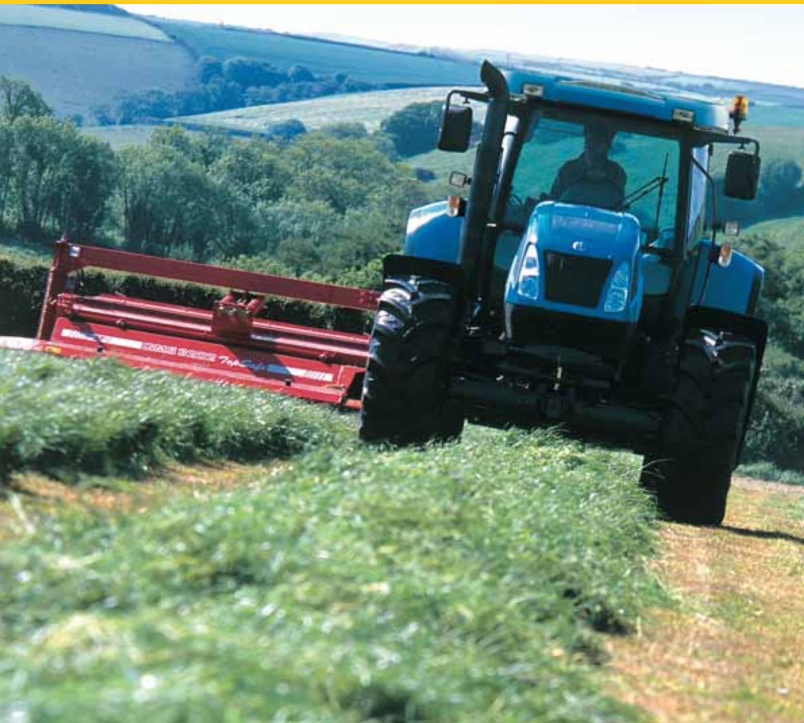
For sheer hydraulic lifting performance Series T7500 is hard to beat, with a maximum lift capacity of 9900kg. Similarly capable of handling the most demanding applications is the advanced load sensing CCLS pump, delivering 105l/min, which can climb to 130l/min when the MegaFlow™ pump is specified. The system is extremely efficient, with precise and rapid pump control for true performance on demand.
