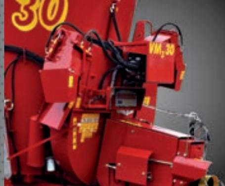
The turbine can be fitted on all versions 2 or 3 augers. Possibility to unloading with the turbine. The turbine is standard fitting with 2 speeds gear-box. Cardan shaft for turbine with clutch and free-wheel.
