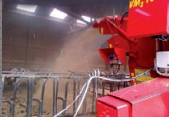
Spreading of straw up to 18 meters.
