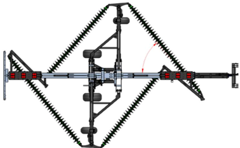
Hydraulic displacement due to aggressive angle of attack (optionally available for a surcharge)
