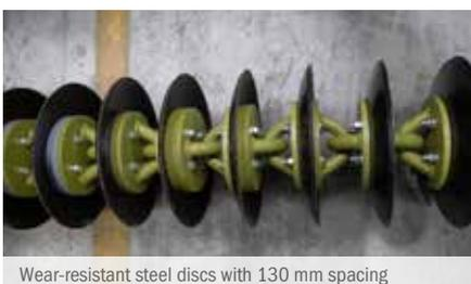
Wear-resistant steel discs with 130 mm spacing
