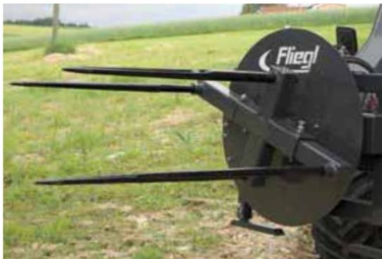
For attachment to Euronorm mounting and three-point hitch
