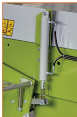
Hydraulic pick up gives precise movement to pick-up system that can work any condition on the field
