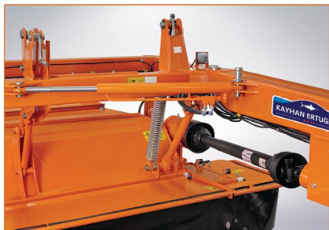
Special suspension system offers flexibility and durability in all field conditions.
