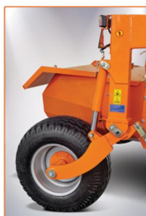
Easy to switch between on road/duty by hydraulic system.
